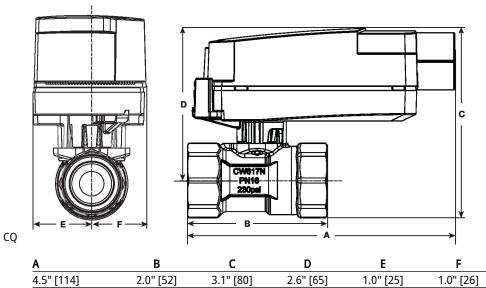
Modulating, Electrical fail-safe, 24 V
